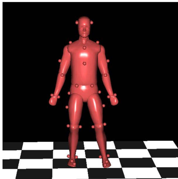
Figure 8.1: Shape Model with the corresponding virtual marker and the pose for the static trial
