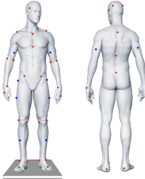
Figure 3.5: Marker Set for the inverse kinematics
