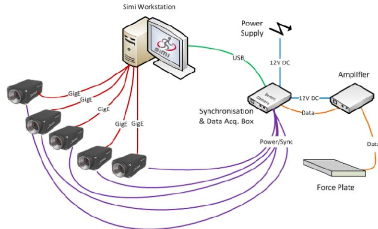
Figure 3.4: schematic setup for a 5-camera-system with integrated force plate
