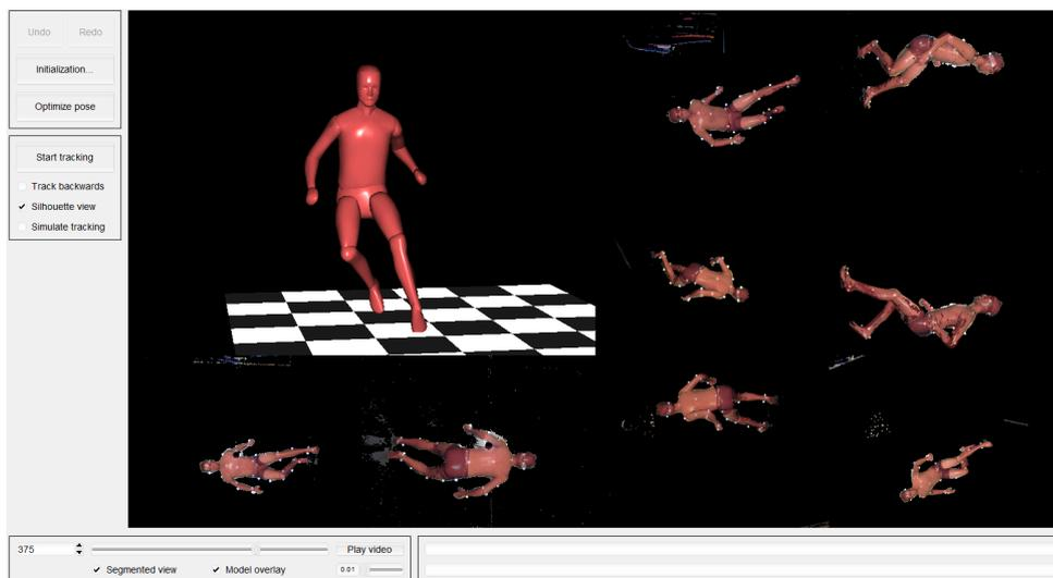
Figure 3.6: Example of a good background subtraction and model fitting in Shape in all eight cameras
