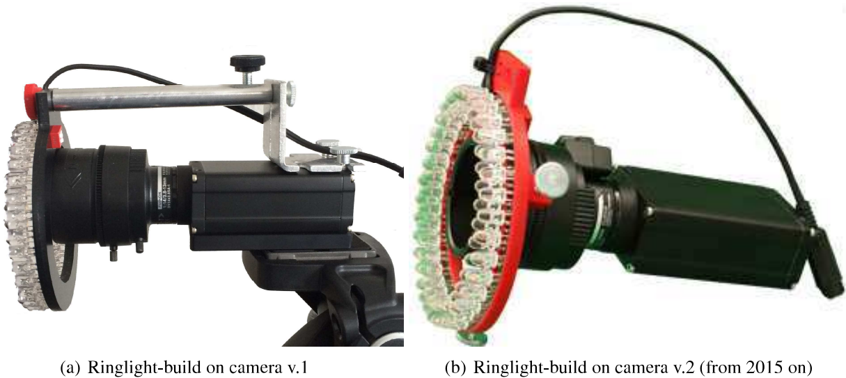
Figure 17.2: Two possibilities of attaching the LED-ringlights
