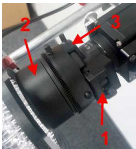
Figure 17.9: 1. Aperture ; 2. Zoom; 3. Focus
