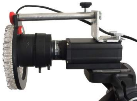
Figure 1.1: Camera with lenses and ring lights [7, p.50]
